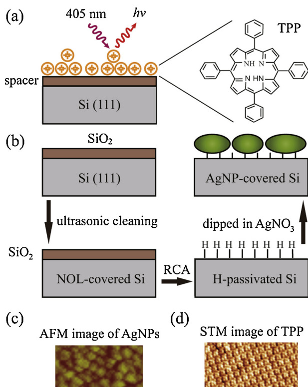
Fig. 1. (a) Schematic of the TPP/Spacer/Si sample with the molecular structure of TPP shown on the right. (b) Schematic flowchart for the fabrication of nanoscale spacers. (c) AFM image (500 nm \times 250 nm) of AgNP film on the hydrogen-passivated Si. (d) STM image (2.5 V, 10 pA, 20 \times 10 nm 2 ) of the first-monolayer TPP molecules on Ag (111).
