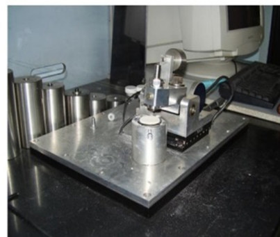
Fig. 2. On the left a schematic of the pin on disk test with the developed forces, on the right the pin on disk equipment.
