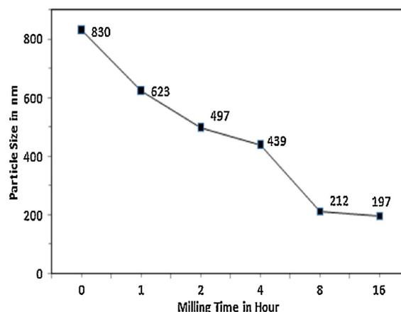
Fig. 1. Effect of milling time on particle size.
