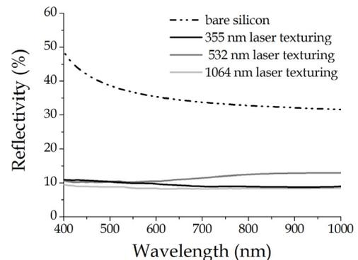
**Fig. 2.** Spectral reflectivity of mc-Si samples textured with 355, 532 and 1064 nm laser wavelengths (without anti-reflection coating, OS = 4). The reflectivity of bare silicon [14] is also shown for comparison.
