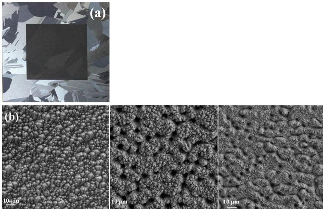
**Fig. 1.** (a) Picture of a textured mc-Si sample; (b) SEM micrographs of Si areas textured with 355 (on the left; OS = 4, peak fluence:  $0.61 \text{ J/cm}^2$ ), 532 (in the center; OS = 4, peak fluence:  $2.18 \text{ J/cm}^2$ ) and 1064 nm (on the right; OS = 4, peak fluence:  $0.97 \text{ J/cm}^2$ ) laser wavelengths.
