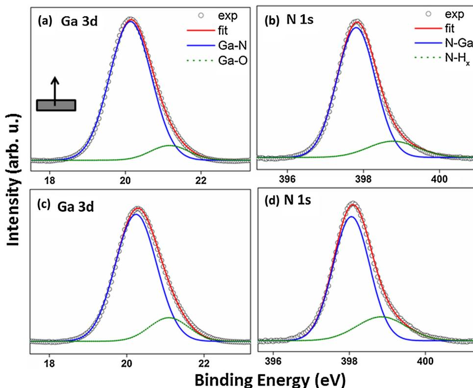
**Fig. 1.** De-convoluted XPS spectra of Ga (3d) core levels of (a) nonpolar and (c) polar GaN film, and N (1s) core level of (b) nonpolar and (d) polar GaN films at TOA = 0°. Open circles showing experimental data while solid lines are fitted curves.
