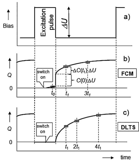
**Fig. 1.** Timing and sampling sequences relevant to the operation modes of ACTP (Advanced Charge Transient Processor): (a) pulsed bias voltage applied to the sample, (b) capacitance measurement in time-domain performed in the FCM mode (Feedback Charge Mode) and (c) isothermal charge DLTS, where the rate window is swept over the charge transient response.
