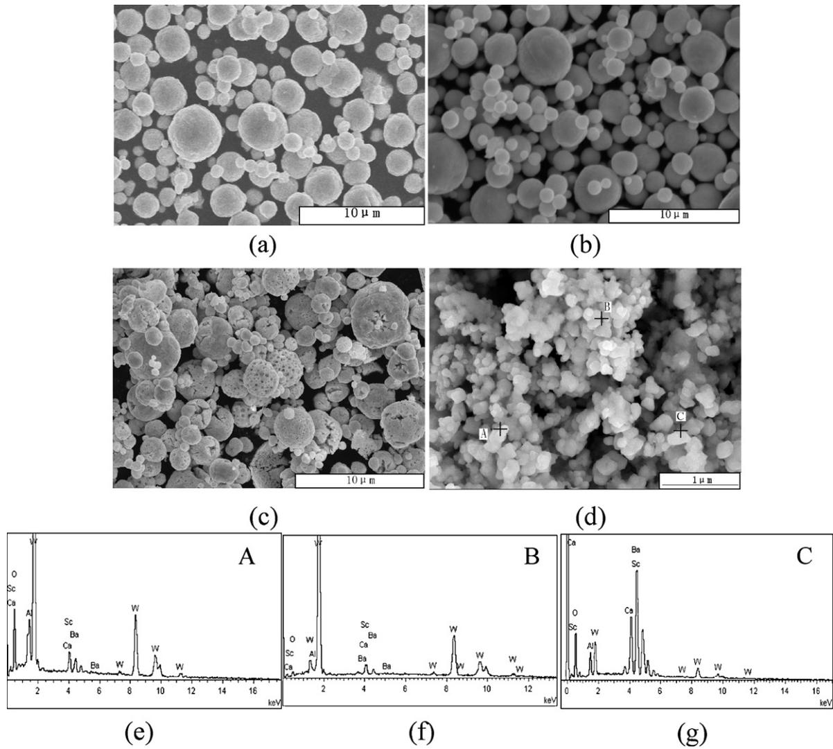
**Fig. 1.** SEM images of (a) pure tungsten oxide powders, (b) scandia and barium–calcium aluminate co-doped tungsten oxide powders, (c) pure tungsten powders prepared with powder (a) through reduction at 850 °C for 1 h, and (d) scandia and barium–calcium aluminate co-doped tungsten powders prepared with powder (b) through reduction at 850 °C for 1 h, (e), (f) and (g) corresponding EDS results of powder (d).
