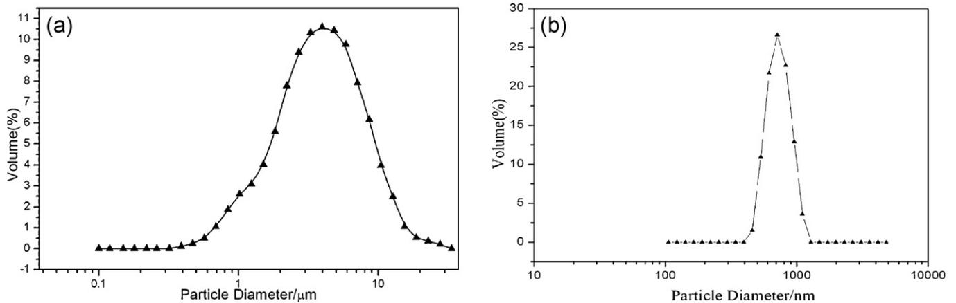
**Fig. 2.** Size distribution curves of (a) pure tungsten powders, (b) scandia and barium–calcium aluminate co-doped tungsten powders.
