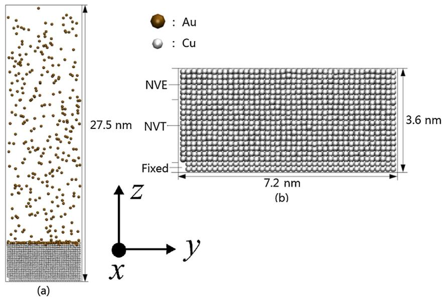
Fig. 1. Simulation model system of deposition. (a) System model. (b) Substrate model.
