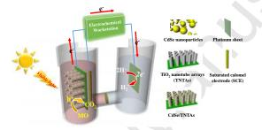
A highly efficient CdSe/TiO<sub>2</sub> nanotube arrays photoanode was explored *via* the electrodeposition with ion-exchange method for photoelectrocatalytic hydrogen evolution and simultaneous degradation of organic pollutant under visible light irradiation.
