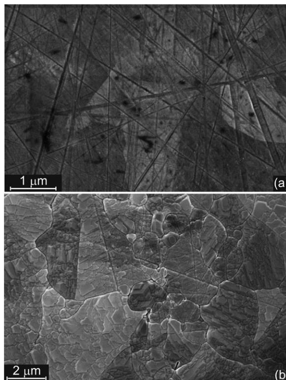
**Fig. 2.** SEM images of CVD polycrystalline SiC samples. (a) An as-received surface before annealing showing many scratch lines due to a mechanical polishing process. (b) A lower magnification image of the sample annealed at 1200 °C for 60 h in vacuum. Significantly fewer scratch marks are visible.
