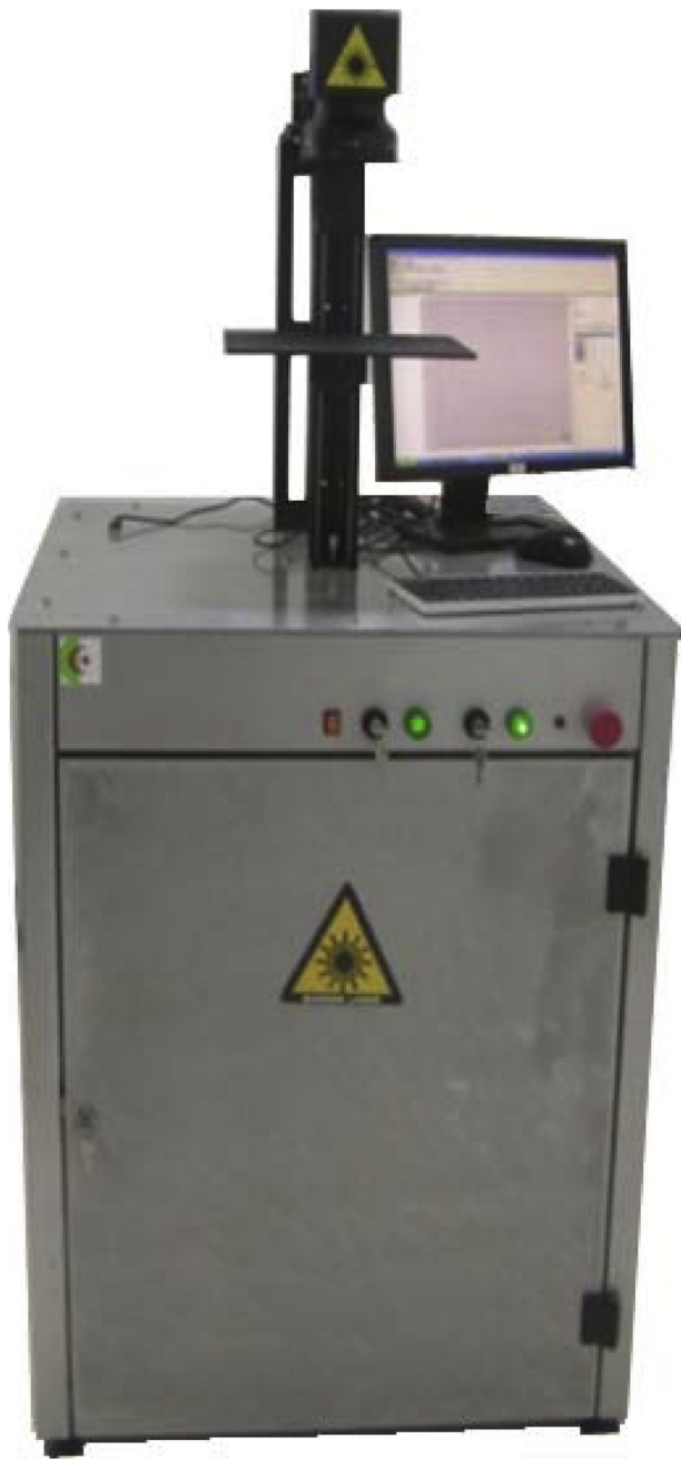
Fig. 1. The used homemade device for metals laser marking.
