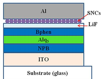
Fig. 1. Schematic device structure of the OLED with SNCs.
