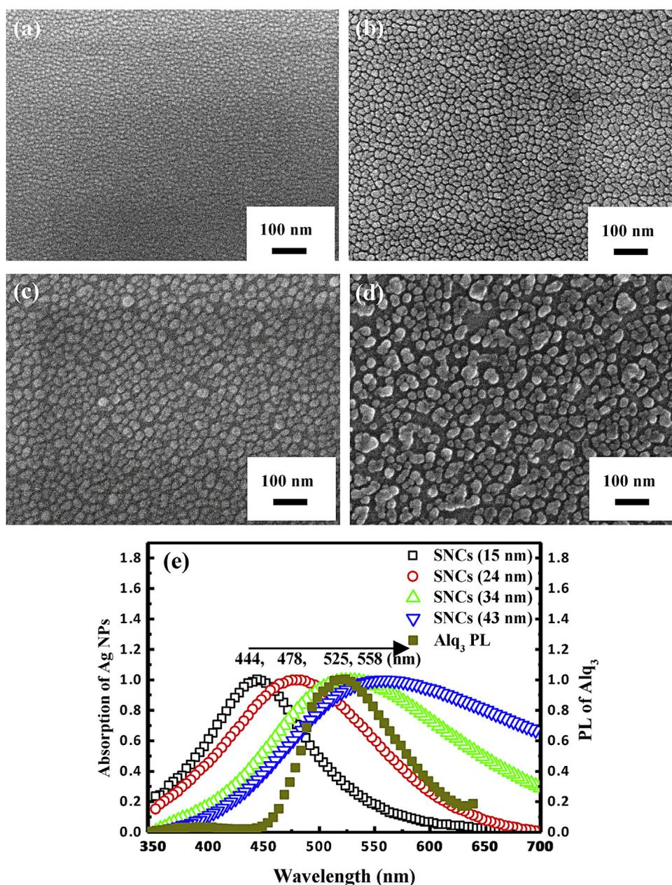
Fig. 2. The SEM images of SNCs at (a) 15 nm, (b) 24 nm, (c) 34 nm, and (d) 43 nm. (e) Normalized absorption spectra of the SNCs with different mean cluster sizes and PL spectrum of the Alq<sub>3</sub>.
