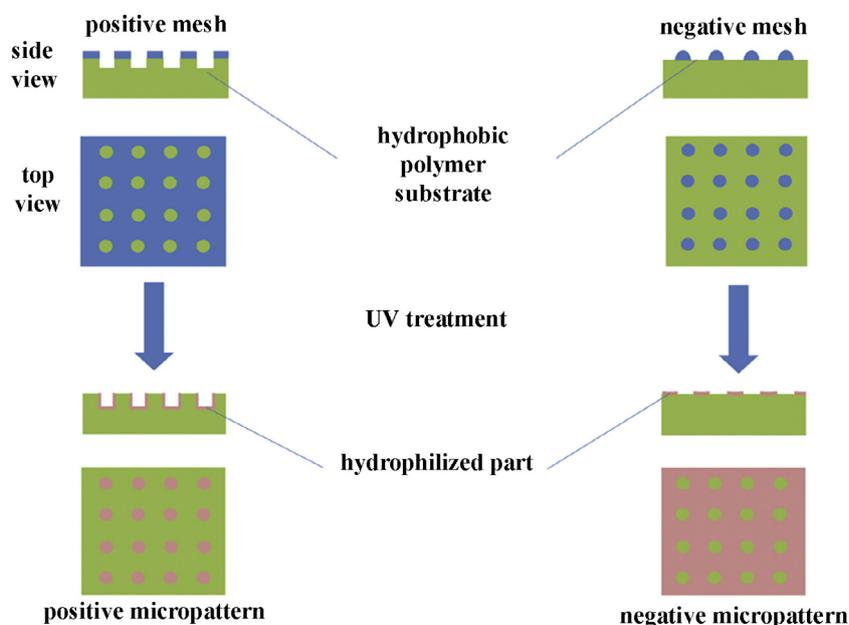
**Fig. 1.** Schematic representation of the positive and negative meshes, and the hydrophilized positive and negative micropatterns. The scheme is not drawn to scale.
