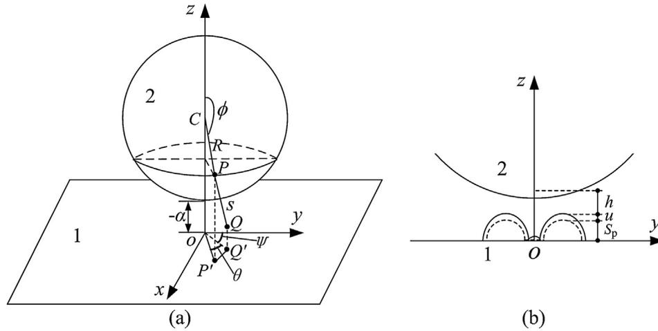
Fig. 1. Adhesive contact between an elastic substrate 1 including surface textures and a rigid sphere 2. (a) 3D plot, and (b) enlarged cross-sectional profile.
