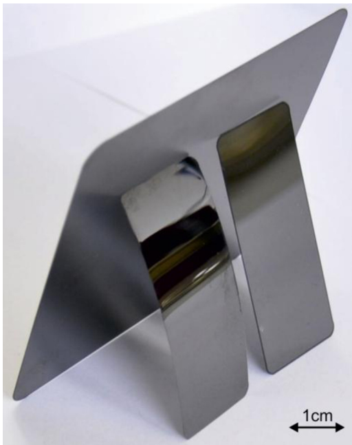
Fig. 1. Photograph of self-supporting nanocrystalline diamond foil building a “house of cards”.
