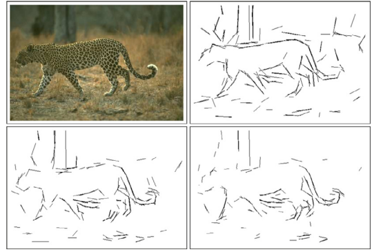
Fig. 1. From lexicographic order: original image number 134052 of the BSDS300 and Line Segment Detection ( N_l = 70 detected straight line segments) at three different resolution levels (namely {0.25, 0.625, 1.0} filtered by the proposed soft edge potential map in the texture sense in order to detect only line segments that delineate the boundaries between different textured areas).
