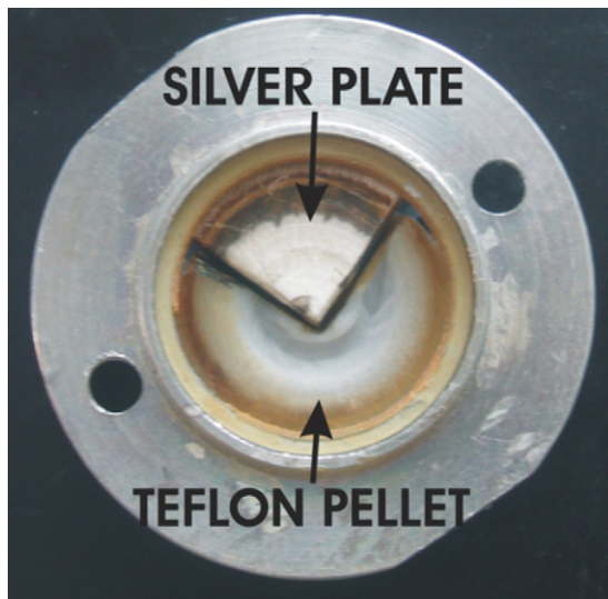
Fig. 1. The ablated target containing 75 vol% PTFE and 25 vol% Ag.
