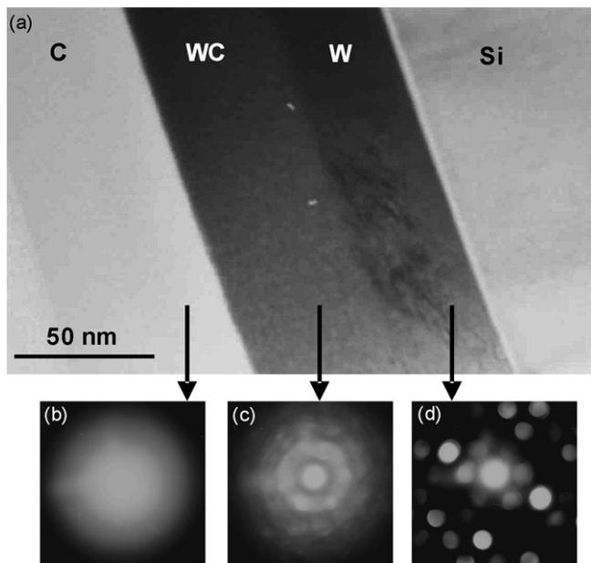
**Fig. 1.** (a–d) TEM micrograph of a cross-sectioned C-graphite (59 nm)/ $W_xC_y$  (50 nm)/W (38 nm) trilayer structure on a smooth silicon substrate (a), and convergent beam diffraction patterns (CBDF) of the C-graphite layer (b),  $W_xC_y$  layer (c) and W layer (d).
