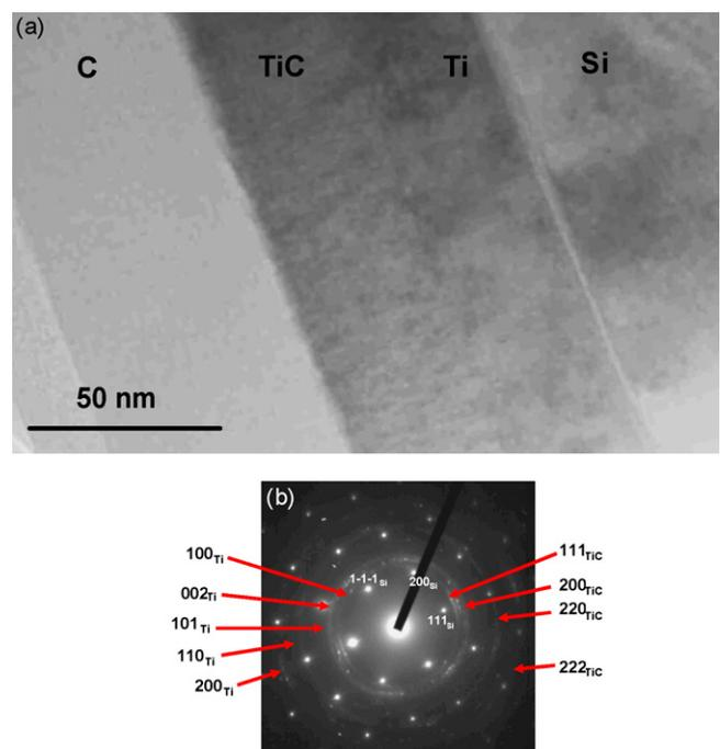
**Fig. 2.** (a and b) TEM micrograph of a cross-sectioned C-graphite (56 nm)/ $Ti_xC_y$  (40 nm)/Ti (34 nm) trilayer structure on a smooth silicon substrate (a), and a selected area electron diffraction pattern (SAED) of the whole region of the C-graphite/ $Ti_xC_y$ /Ti trilayer on the Si substrate (b).
