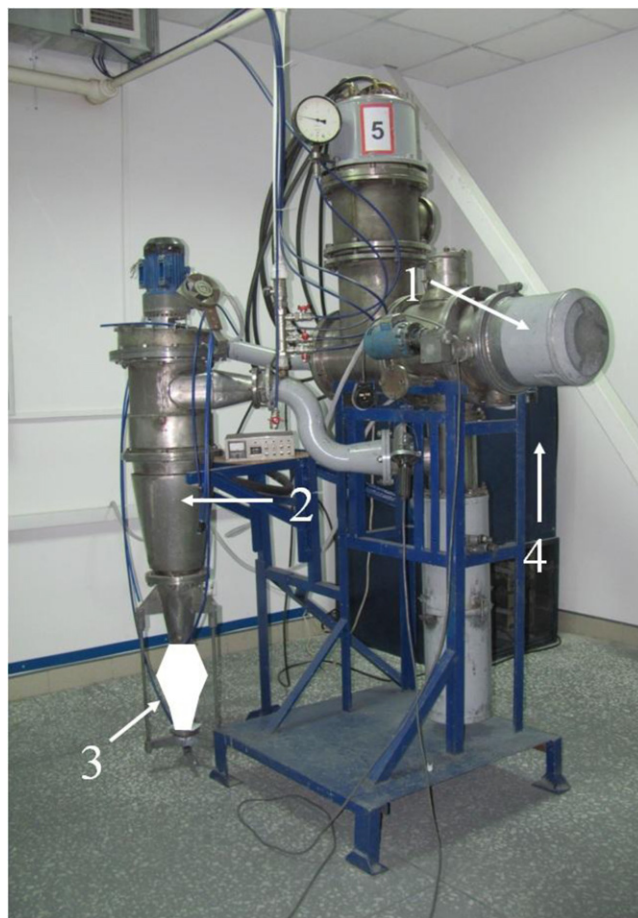
Fig. 1. UDP-5 machine for nAl production with the electrical explosion of wires technology: 1 – explosion chamber; 2 – powder deposition system; 3 – powder collector scheme (not installed); 4 – high voltage unit.
