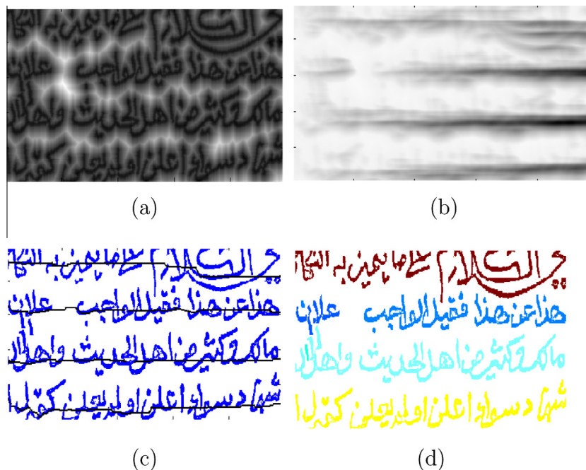
Fig. 1. (a) Calculating a signed distance map, (b) calculating the energy map of all different seams, (c) finding the seam with minimal energy cost, and (d) extracting the components that intersect the minimal energy seam.
