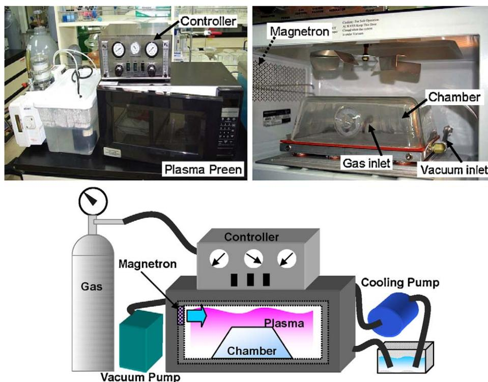
Fig. 1. Photograph and schematic diagram of the plasma apparatus.
