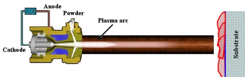
Fig. 1. Schematic of plasma spray torch with a radial powder injection system.
