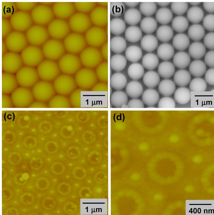
Fig. 1. (a) AFM image of nanosphere lithography (SPL) mask, (b) SEM image of nanosphere lithography (NPL) mask, (c) AFM image of hexagonal pattern nanodots and microrings of fluorinated hydrocarbon, (d) zoomed view of (c).
