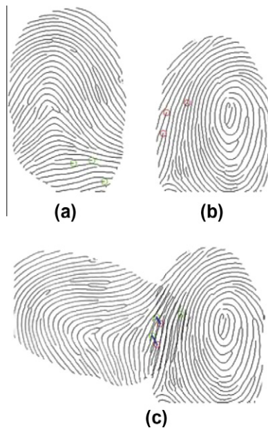
Fig. 1. An example of two fingerprints from FVC2002 DB1. Minutiae from different regions of different fingers are matched very well. The circles denote the matched minutiae: (a) thinned image of 56_1.tif; (b) thinned image of 98_1.tif; (c) registration of (a) and (b).
