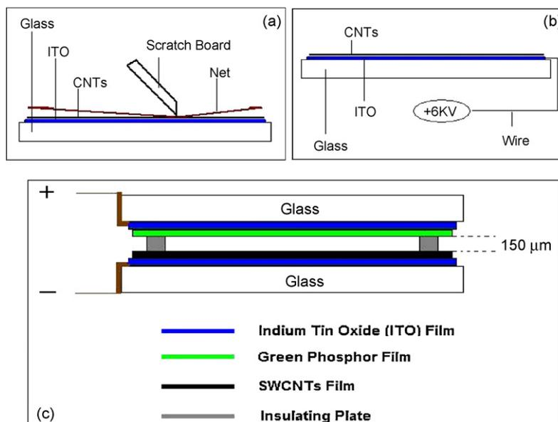
Fig. 1. The fabricating process of cathode and anode plate (a and b); (c) is the structure of FED.
