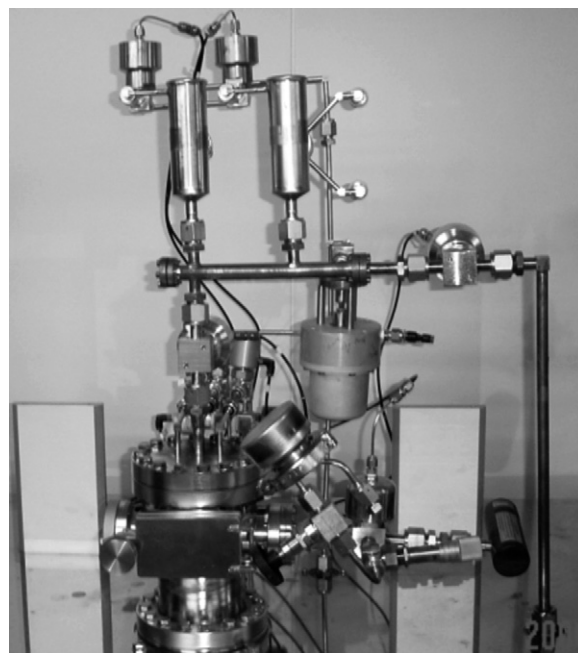
Fig. 1. The experimental plasma enhanced atomic layer deposition system.
