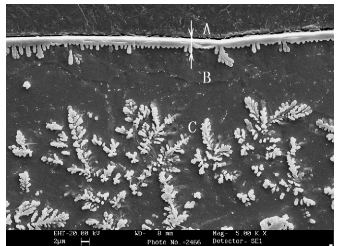
Fig. 2. Cross-section microstructure of LGN NiTi.
