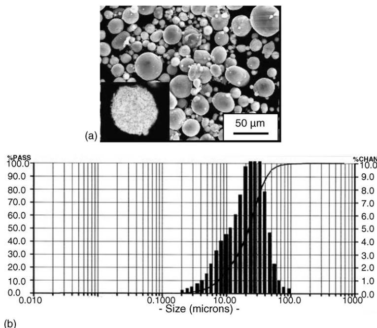
Fig. 1. Feedstock: Al–Si (wt.% 78:12), spherical, +5 to 45  $\mu$ m (mean size 25  $\mu$ m): (a) SEM micrograph of Al–Si powder morphology; (b) laser scatter value of Al–Si powder size distribution (volume fraction).
