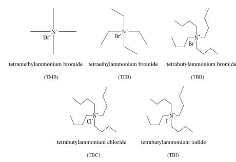
Fig. 1. Chemical structure of alkyl quaternary ammonium halides.
