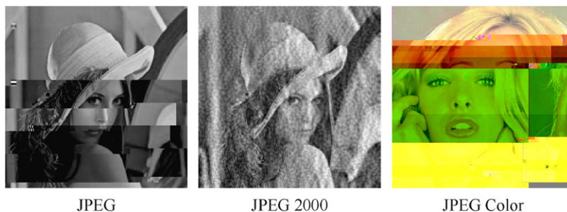
Fig. 1. Images reconstruction when BER is about 10^{-4} and file header not corrupted.
