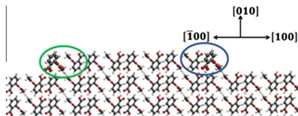
**Fig. 1.** Top view of the stable kink structure at the [010] step edge of the aspirin (001) face. For clarity only the terrace top layer above the step edge is displayed and (green and blue) circles highlight the considered dimeric dissolution unit at the two (inequivalent) kink sites shown. C, O, and H atoms are shown as grey, red and white spheres, respectively. The slowly detaching kink molecules are shown with bold spheres.
