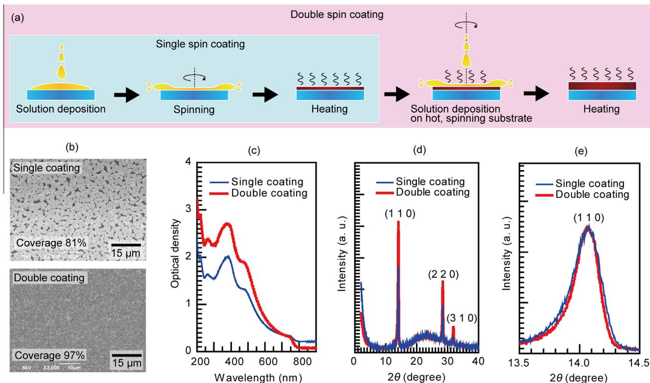
Fig. 1. (a) Schematic illustrations of the single and double spin coating processes. (b) SEM images, (c) absorption spectra, and (d) XRD patterns of single- and double-coated perovskite films. (e) Magnified, normalized XRD patterns from (d).
