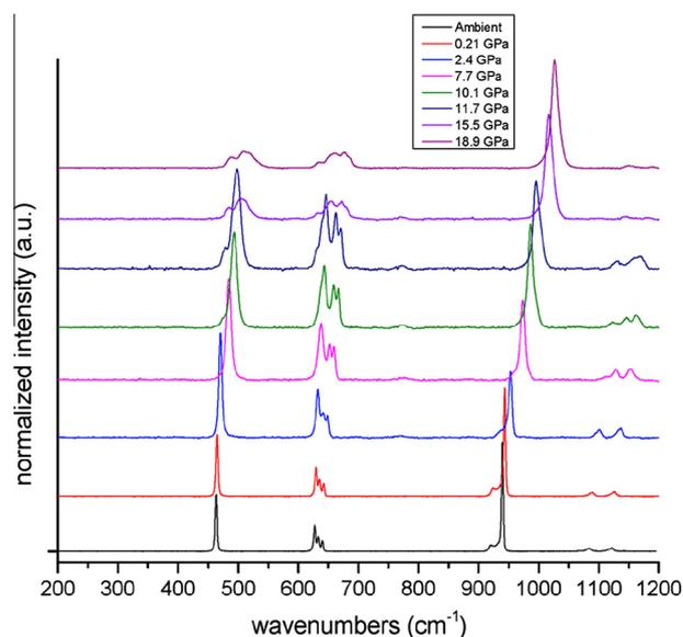
Fig. 1. Raman spectra of  $\text{KClO}_4$  as a function of pressure in the low wavenumber region ( $200\text{--}1200 \text{ cm}^{-1}$ ). New peaks emerge in the 2.4 GPa and 7.7 GPa plots suggest a sluggish phase transition that commences near 2.4 GPa and ends around 7.7 GPa. Above 11.7 GPa, some (not all) of the Raman spectral modes are considerably broadened.
