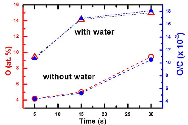
**Figure 3.** Oxygen atomic percentage (left) and oxygen to carbon atomic ratio (right) of the samples after the plasma treatment with and without water.
