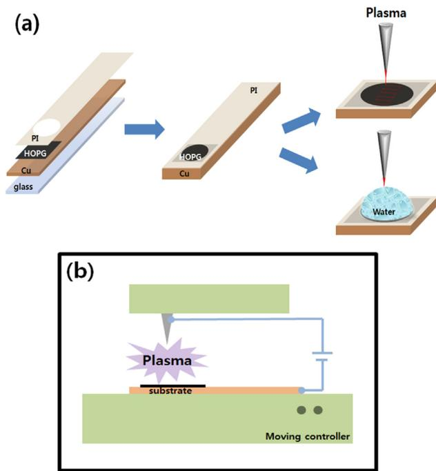
**Figure 1.** The schematics of (a) sample preparations and (b) an experimental setup for the plasma treatment.
