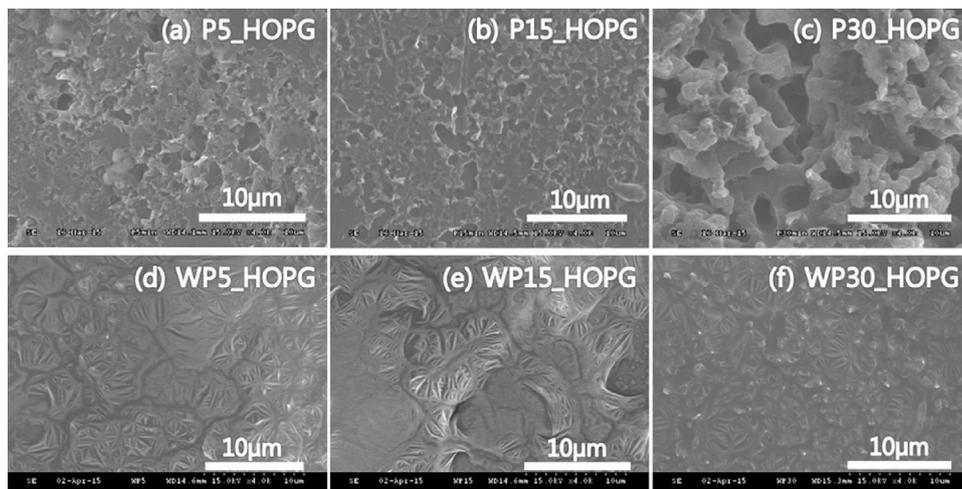
**Figure 2.** SEM images of HOPG samples without water after the plasma treatment for (a) 5, (b) 15 and (c) 30 min, and with water for (d) 5, (e) 15, and (f) 30 min.
