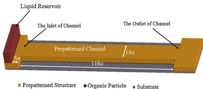
**Figure 2.** Setup of simulation box. The gray balls represent the substrate, the yellow balls stand for prepatterned structures, and the brown balls reflect the organic particles.
