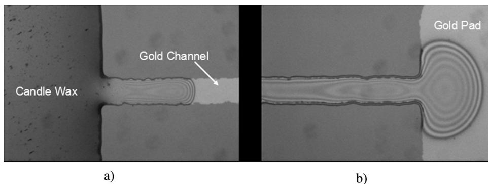
**Figure 1.** Optical microscope images of candle wax on Au patterned SiO<sub>2</sub> with different time. (a) 18 s, and (b) 210 s. The time 0 s is set when the liquid starts to fill the channel.
