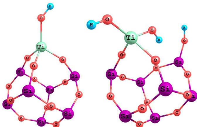
**Figure 1.** (Left) Model for monomeric titania species on silica with three anchoring Ti–O–Si bonds (Model A). (Right) Model for mono monomeric titania species on silica with two Ti–O–Si bonds (Model B).
