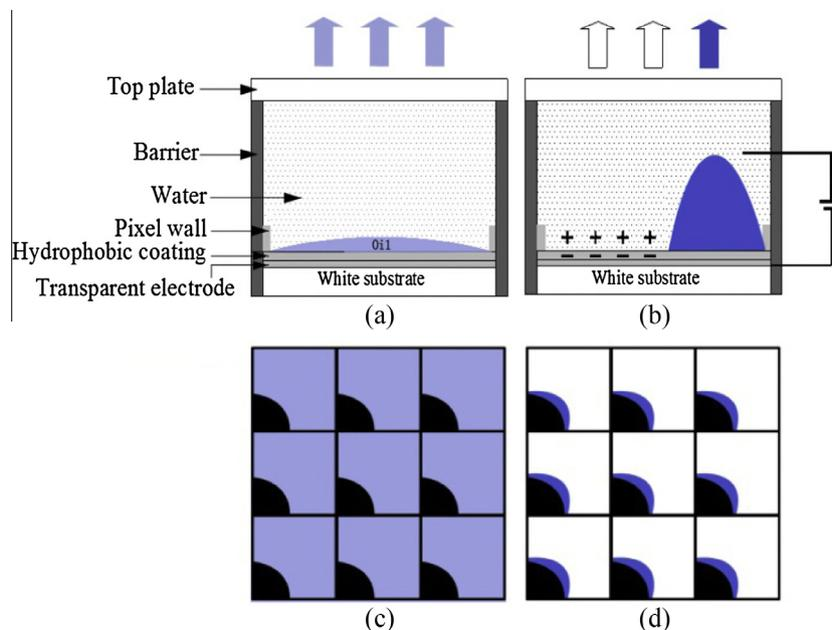
**Fig. 1.** An EWD pixel – principle and components. (a) Side view of electrowetting pixels when the oil is rolled out; (b) side view when the oil is pushed aside; (c) top view when the oil is rolled out; (d) top view when the oil is pushed aside (NB: oil thickness and droplet size not to scale).
