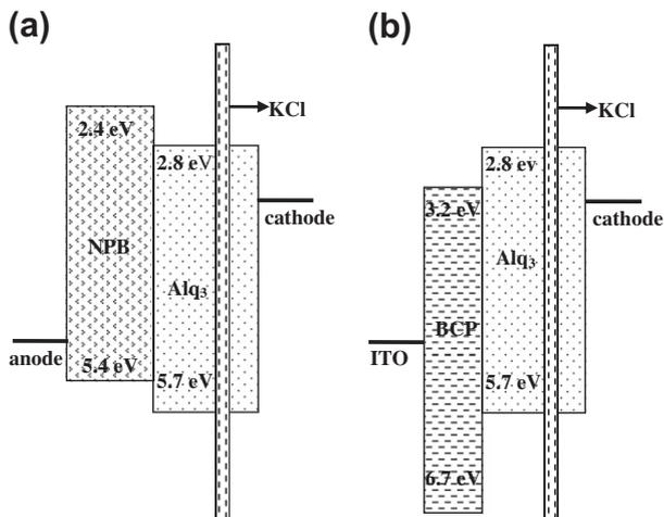
**Fig. 1.** The configurations and the energy level diagram of devices in the experiment. (a) EL devices: **anode**/NPB(40 nm)/Alq<sub>3</sub>(60-*d* nm)/KCl(1 nm)/Alq<sub>3</sub>(*d* nm)/**cathode**. (b) Electron-only devices: ITO/BCP(15 nm)/Alq<sub>3</sub>(60-*d* nm)/KCl(1 nm)/Alq<sub>3</sub>(*d* nm)/**cathode**. Herein, *d* = 10, 20 and 30.
