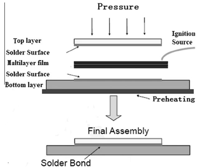
Fig. 2. Schematic of SPER joining process: stacking base materials with preheating and applied pressure.
