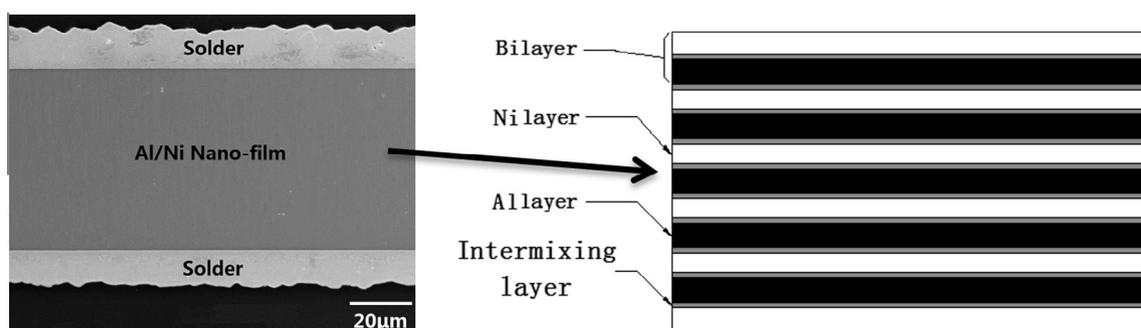
Fig. 1. Al/Ni nano-films used in the SPER: cross-sectional SEM image and the schematic illustration of the multi-layered structure.
