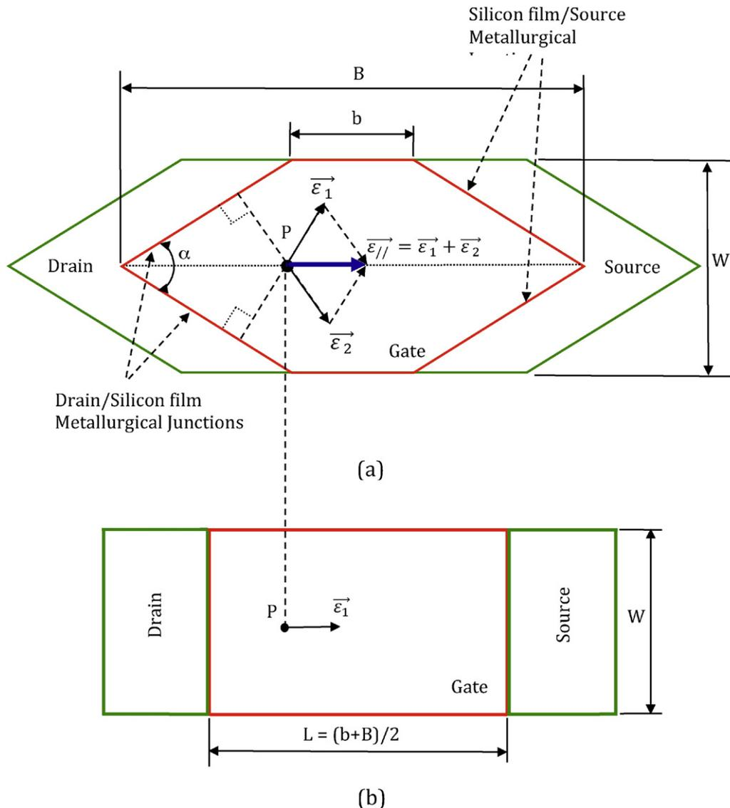
Fig. 1. The simplified top views of the Diamond (a) and its Conventional counterpart (b), regarding the same gate area,  $W$  and its corresponding LEF vector components.
