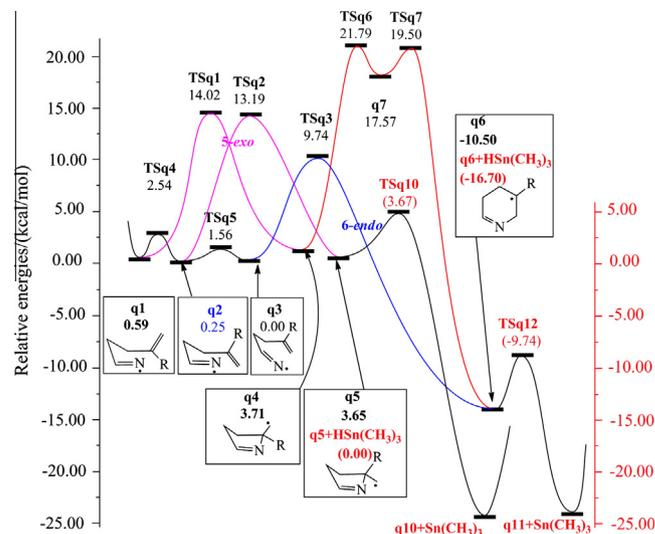
**Fig. 1.** Reaction potential energy profile of system **1q** ( $R = -COOH$ ). For the radical cyclization reactions, the reference zero is reactant **q3**. For the reduction reactions of 5-*exo* and 6-*endo* cyclic radicals (red part), the energy of **q5**+ $HSn(CH_3)_3$  is taken as the energy zero point. (For interpretation of the references to colour in this figure legend, the reader is referred to the web version of this article.)
