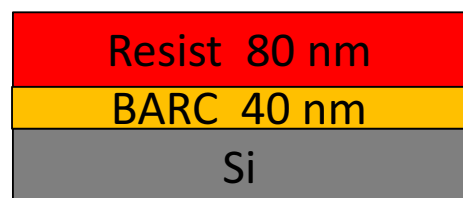
Fig. 3. The substrate to which the pattern is transferred is assumed to have the layers.
