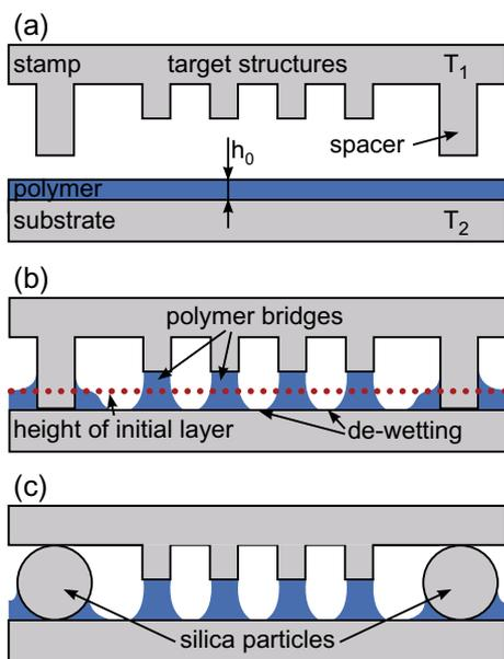
**Fig. 1.** Schematics illustrating the principle of a process forming isolated polymeric bridges with a 3-level stamp. (a) Before the process. (b) After the process. Initially there is a gap between the elevated stamp structures and the initial layer. Finally the polymer builds isolated bridges between stamp and substrate. (c) Realisation with 2-level stamp; silica particles were used as spacers.
