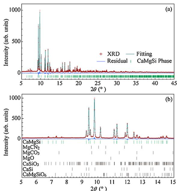
**Fig. 1.** Synchrotron radiation X-ray powder diffraction patterns (cross symbol) of wide (a) and narrow ranges (b) for CaMgSi compound at 300 K. The thin line, dots, and vertical bars indicate the fitting, residual, and CaMgSi phase results, respectively, calculated by Rietveld analysis. (For interpretation of the references to color in this figure legend, the reader is referred to the web version of this article.)
