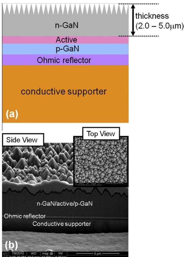
Fig. 1. (a) The schematic diagram of GaN-based vertical LEDs and (b) scanning electron microscope (SEM) images of a vertical LED chip.
