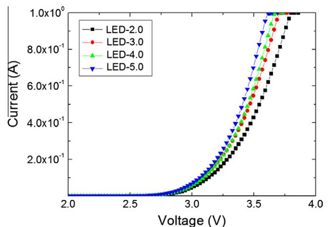
Fig. 2. The typical forward current–voltage ( $I$ – $V$ ) characteristics of vertical LEDs as a function of the n-GaN thickness.
