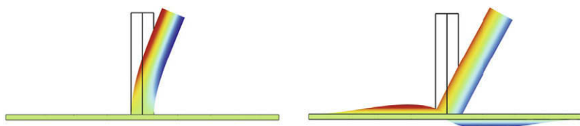
Fig. 2. Finite element simulation of the first flexural eigenmode of a silicon column on (a) a rigid silicon substrate and (b) a 2 \mu\text{m} thick silicon nitride membrane clamped at the circumference. The dimensions are in accordance with the geometrical data of the sensors from the SEM image in Fig. 1 and optical image in Fig. 5, respectively.
