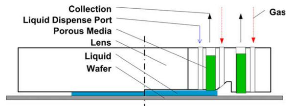
**Fig. 3.** Schematic of the immersion unit.
