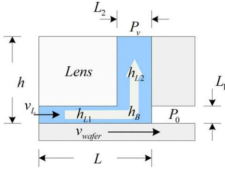
**Fig. 1.** Schematic of the important parameters that affect noncontact sealing boundaries. While wafer is moving, the liquid is injected and collected to maintain the optical uniformity beneath the stationary lens.
