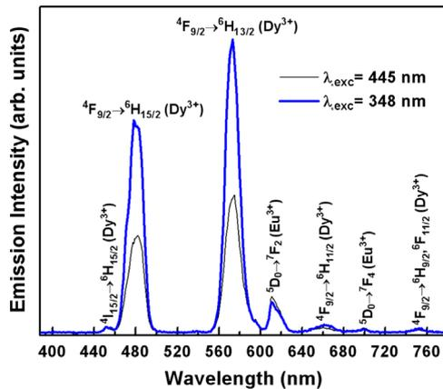
Fig. 1. Emission spectra of the ZPEuDy glass excited at 348 and 445 nm.
