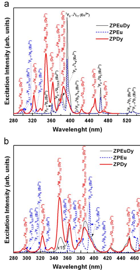
Fig. 2. (a) Excitation spectra of the glasses ZPEuDy ( $\lambda_{em}=615$  nm), ZPEu ( $\lambda_{em}=615$  nm) and ZPDy ( $\lambda_{em}=573$  nm). (b) Excitation spectra of the glasses ZPEuDy ( $\lambda_{em}=480$  nm), ZPEu ( $\lambda_{em}=615$  nm) and ZPDy ( $\lambda_{em}=573$  nm).
