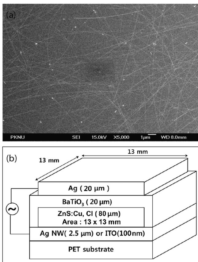
Fig. 2. (a) Top-view SEM image of Ag nanowires and (b) schematic of EL device.
