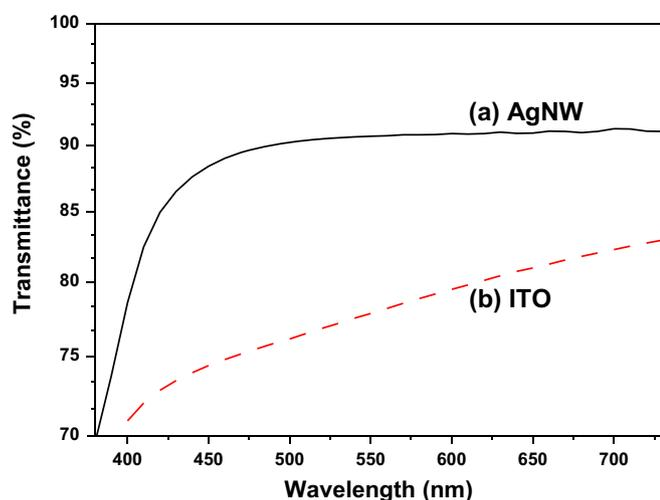
Fig. 1. Transmission spectra of (a) Ag nanowires and (b) ITO PET substrates.
