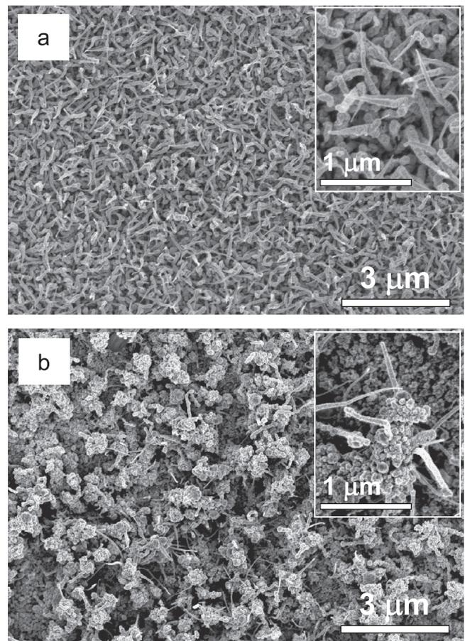
**Fig. 1.** FESEM images of Si/SiC core-shell nanowires prepared by HWCVD at different deposition pressures of (a) 0.5 and (b) 1 mbar. Insets of each figure present a high magnification of the respective FESEM images.
